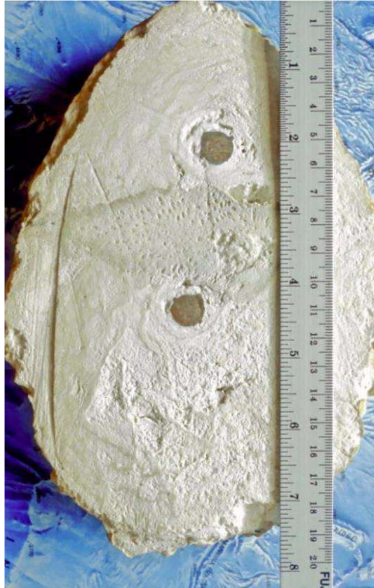
Mineral accretion sample from Maldives which was grown electrolytically during only five years.
